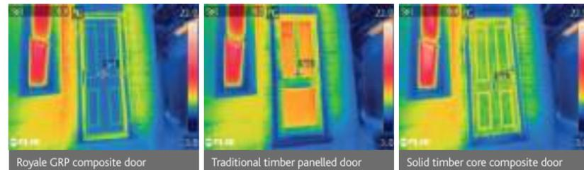
**19%** more thermally efficient than a 48mm solid timber core composite door
